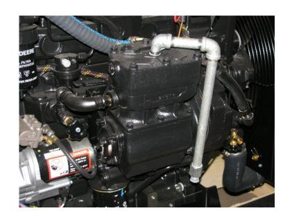
Direct drive 2 cylinder piston air compressor producing 15 cfm @ 90 psi with 125 psi max.
