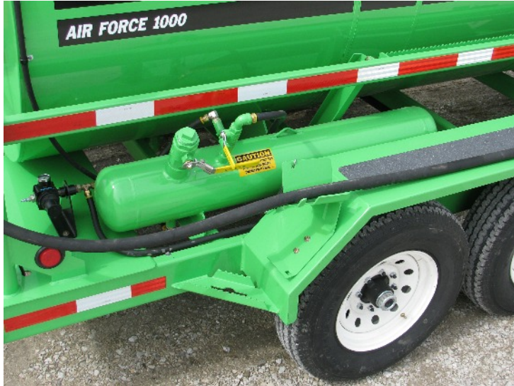
Clean out tank
