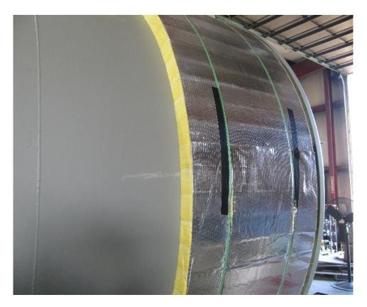
3" High density foil backed insulation blanket completely covers the tank to prevent heat loss.
